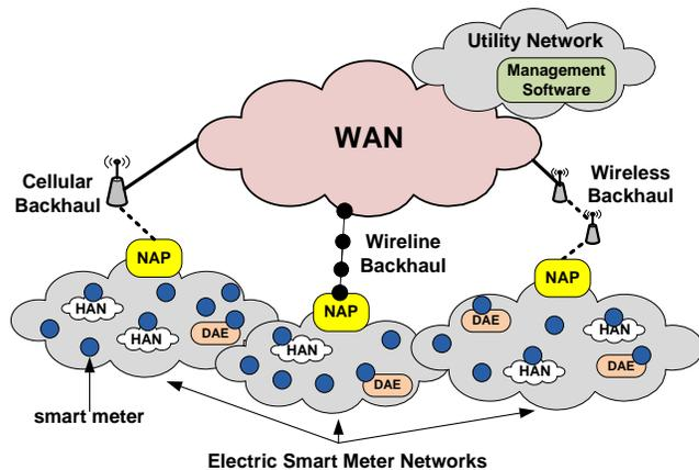
Figure 1: Smart Grid Network Example. Acronym definitions: HAN (Home Area Network), DAE (Distribution Automation Element), NAP (Network Aggregation Point), WAN (Wide Area Network).
