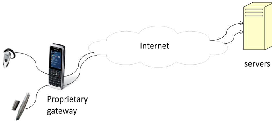
Figure 1 Sensors connecting to Internet server without IP
