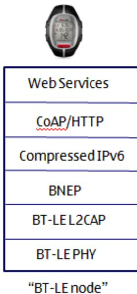
Figure 3 IPv6 over BT-LE, complete stack in the sensor
