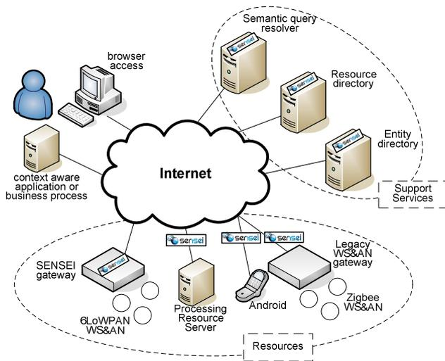
Figure 1. SENSEI testbed
