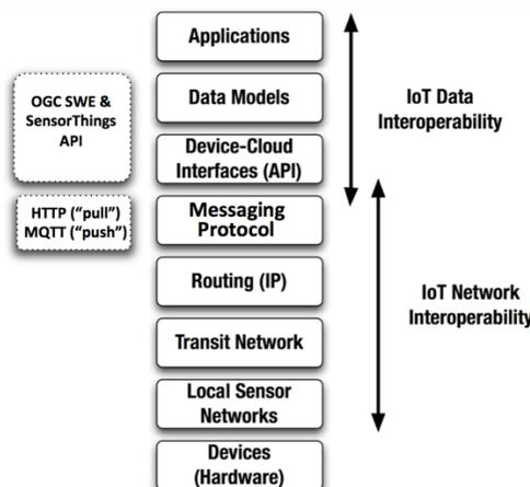
Figure 2 A Layer Diagram of the IoT Interoperability Layers
