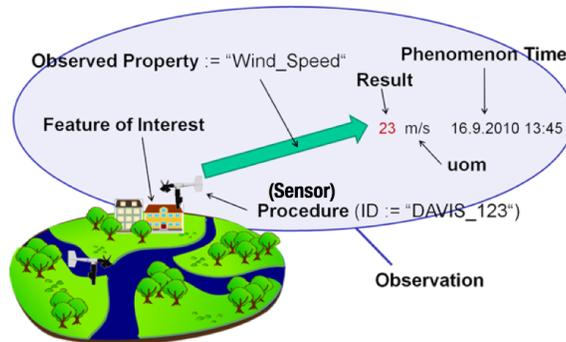
Figure 1 Relationships between the entities of the OGC/ISO Observation and Measurement Data Model
