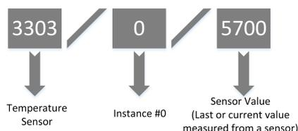
Fig. 1. Temperature Sensor URI Example.
